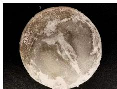
Circumferential cracks appeared but no visible spalling, PC, 150d
