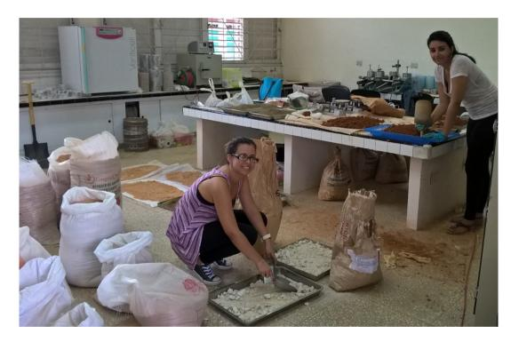
Fine and coarse aggregates were sieved and prepared to comply with Cuban standard NC 251
