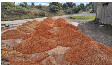
Calcined Clay ready to be milled (produced in Ranville cement plant, North of France)
