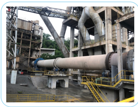
Illustration of clay calcination using rotary kiln (left – Ciplan Brazil) and flash calcination (right – Vicat France).
